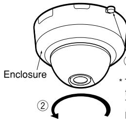
① Remove the fixing screw.
